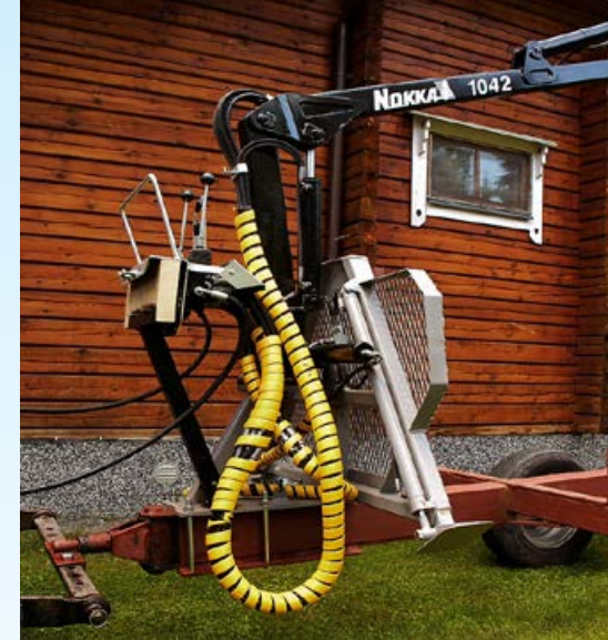
Loader mounting on self-made trailer by mounting device module.
