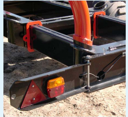
Telescopic frame extension and lighting device
