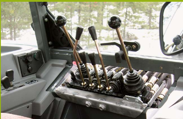
Mechanical 2-lever valve block in the cabin. (Std)
