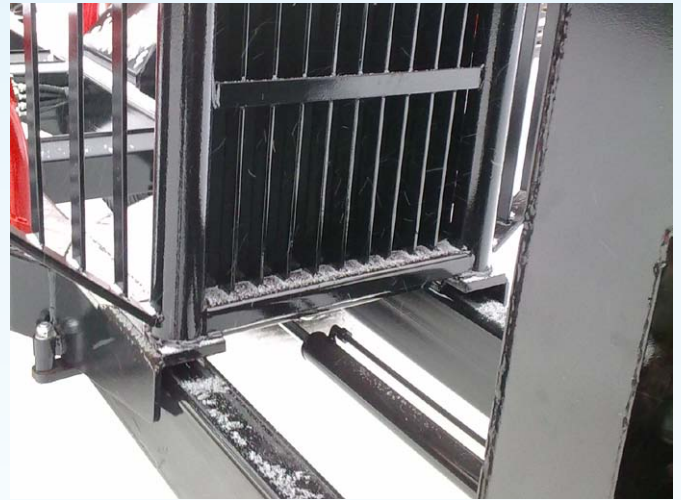
Hydraulically movable front screen (only for factory setting).
