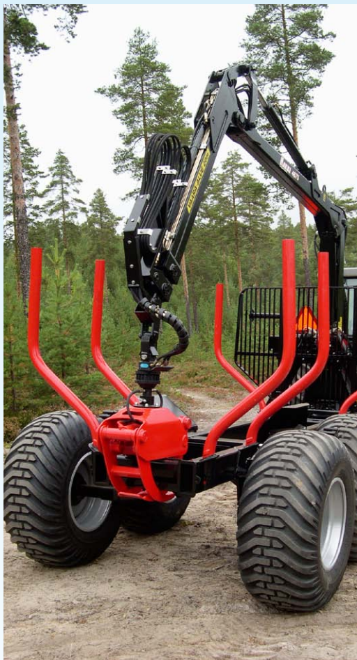
100-series forest trailer has good ground clearance and many tyre alternatives.
