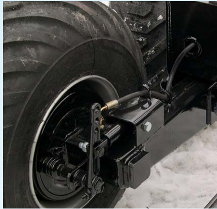
Hydraulic brakes on one and two axle.
