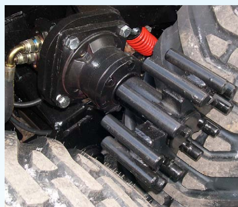
The non-skid drive is due to specially ribbed tires which adjust like a gear type connection between the drive rolls and the tires.
