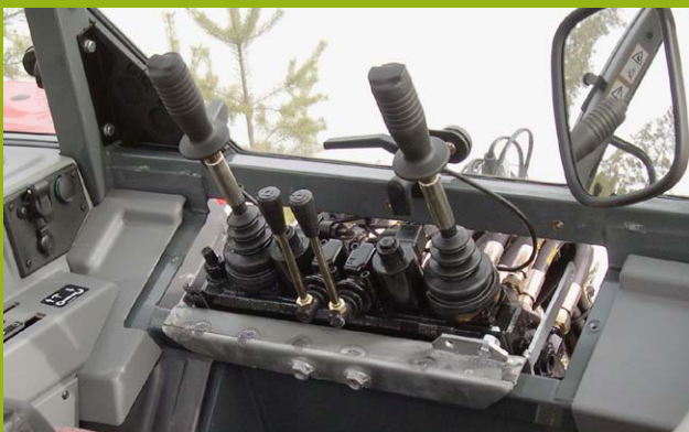
On/off 2-lever valve block (He). Hydraulic extension and grapple used electrically. Valve block mounted in the cabin.
