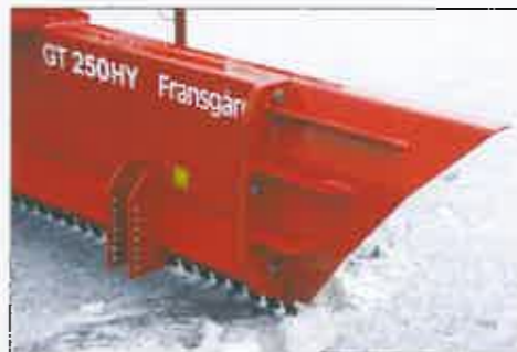
The snow wing is puts a finishing touch to snow removal. The wing creates an angle on the snow edge preventing the snow from sliding back down.
