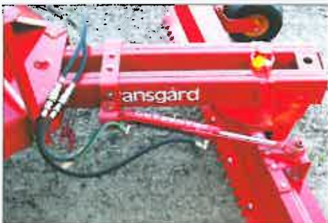
A hydraulic toplink with attachment brackets is available for blade adjustment.
