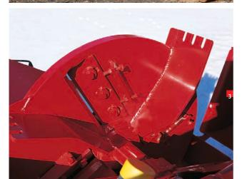
The HJ-260 is a direct feed chipper for wood 25 cm in diameter. It is well-suited for producing biofuels and woodchips used as energy sources and in stoker boilers. The high-quality woodchips produced with direct feed chippers is particularly well-suited for use in stoker boilers, since the chipper cuts the wood to the cross fibre. The feed opening is at a 90 degree angle to the blade disk.
