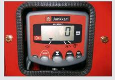
No Stress control Wizard C. The rotational guard of the manual feed chipper also features other practical functions such as an hour counter and a maintenance alarm.
