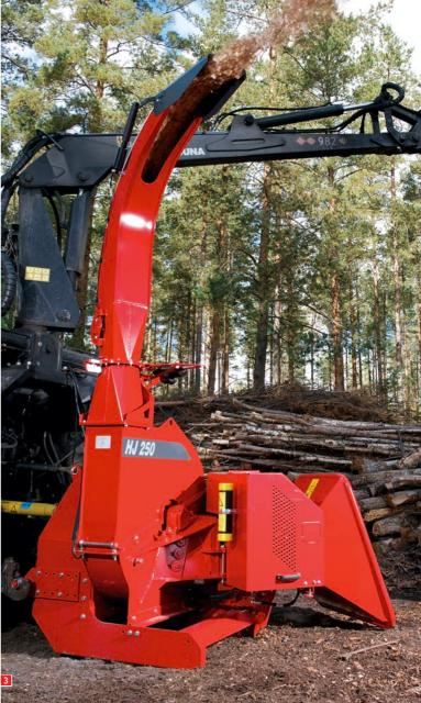
1 The HJ-250 G model is a chipper with a hydraulic feeding device. Its two feed rollers are powered by the tractor's hydraulics. The HJ-250 GT model is almost identical to it: the only difference is that its feeding device has an independent hydraulic tank and pump. This means that no additional hydraulics is needed.
