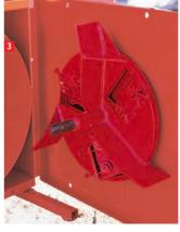
The three blades of the disc can be adjusted continuously to the desired woodchip size. The blow wings will finalise the woodchips and blow the chips effectively to the desired location through an adjustable discharge chute.
