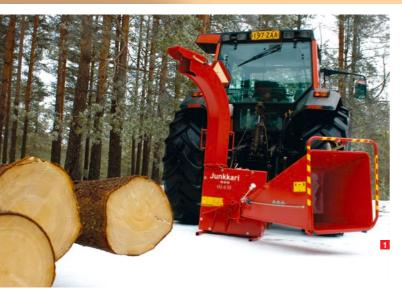
Junkkari's smallest HJ-4 chipper is ideal for environmental chipping and landscaping. It is a nondirect feeding chipper. The blades draw the wood in themselves, and it requires less power. The HJ-4 chipper comes in two versions, the M and the G models. The HJ-4 chipper can be used to chip wood with a diameter of up to 9 cm.
