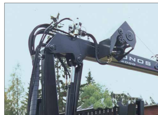
Radio controlled hydraulic winch. 1400 kp, wire: Ø 6 mm, length 35 m
