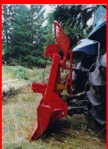
the top pulley provides additional resistance when pulling heavier logs
