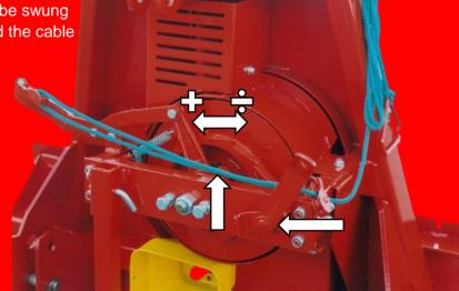
Cable drum **locking latch** will prevent unwanted backwards movements of the log
